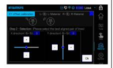
4. Click the +/- button to input the calibration value. Check the print model and set the appropriate compensation value, then click the **OK** button.
