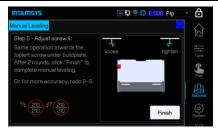
M6. After the second pass of manual leveling is completed, click Finish button, the platform will drop to the bottom, and then return to the end of manual leveling.
