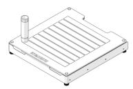
2. Use a solid glue stick to evenly apply 4 layers of primer to the printing area of the printing glass buildplate to increase the adhesion of the first layer during printing.
