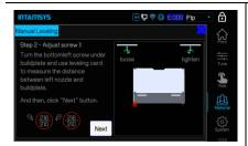
M4. According to the prompts on the screen, rotate the knobs under the printing platform by hand, and use a leveling card (thickness 0.2mm) to measure the distance between the nozzle and the glass plate of the platform. Then click the **Next** button.
