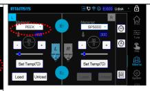
3. Click the **Drop-down** menu to select the filament. Make sure that the filament you select is the same as the filament you want to load. Click **Set Temp** to heat the nozzle to the set temperature.
