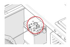
Cleaning the filaments chamber: The frequent contact between the feed gear of the auxiliary wire feeding mechanism and the filament produces debris. Use a sharp needle to clean the debris at the gap of the gear, then use a vacuum cleaner to clean up the debris of the filament, and wipe the residual dust with a cleaning cloth and alcohol.
