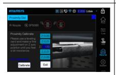
A4. Use a leveling card(0.2mm thickness) and click "Z10.05" or "Z10.05" to make preliminary adjustments, and click "Z10.01" or "Z10.01" to make fine adjustments, the distance between the nozzle and the buildplate just put in the card.
