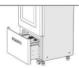
1. The material silo is located in the lower half of the printer. Push the silo door forward, and the silo will pop up automatically. Push the transparent top door of the silo forward to open the material silo.
