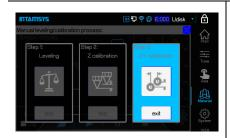
1. Calibrate the deviation of the left and right nozzles in the X and Y directions, the deviation value is obtained by actually printing the calibration model. Click XY Calibration to enter the sub-
