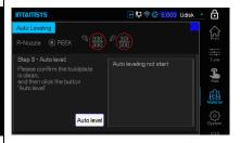
A6. The screen prompts to clean the printing platform. If it has been cleaned up, click the **Autolevel** button to prepare for the official implementation of automatic leveling;
